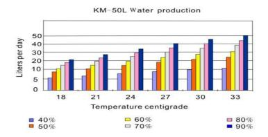
For example; in the above chart where the average humidity is 60% (yellow bar) and at a temperature of 24 ° Celsius the anticipated water production from a 50 litres machine is 20 litres per day. WHEREAS if the temperature rises to 33° Celsius the anticipated water production rises to 30 litres of water at the same humidity level.
